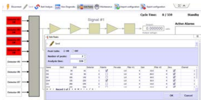
Figure 4 - programming 4 optical sensors in one PlasmaDetect-2 detector
