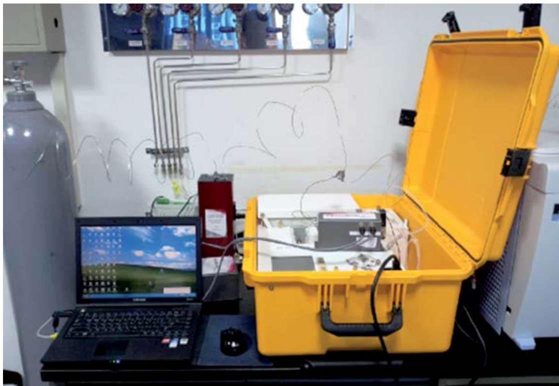
Figure 5: PlasmaDetek installed in a portable unit
