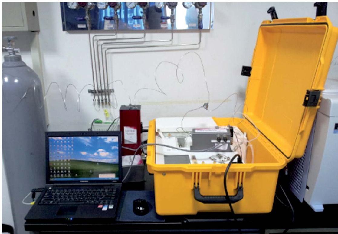
Figure 5: PlasmaDetek installed in a portable unit
