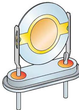
Figure 1: Quartz crystal sensor
