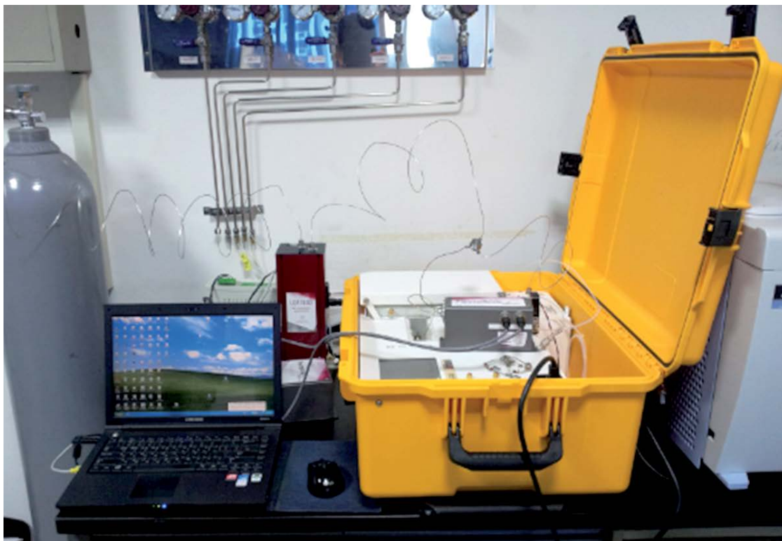
Figure 5: PlasmaDetek installed in a portable unit
