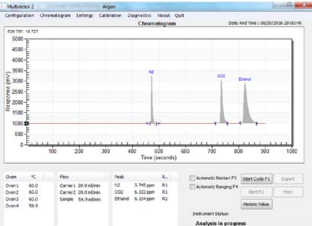
Span calibration chromatogram for Argon method:
