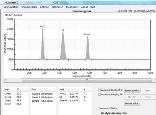
Span calibration chromatogram for Carbon dioxide method:
