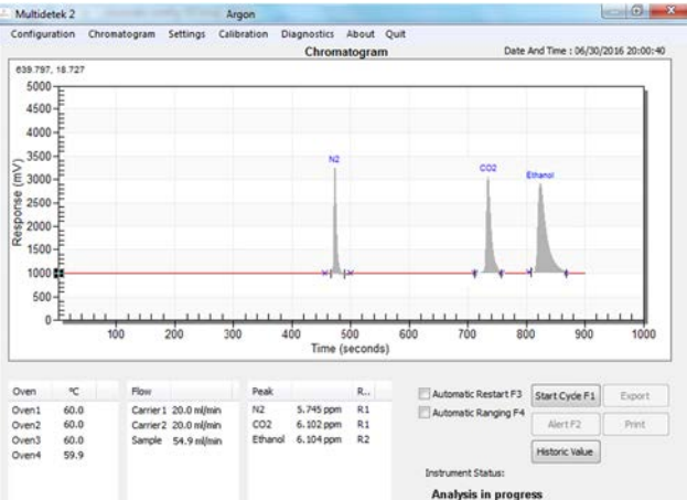
Span calibration chromatogram for Argon method:
