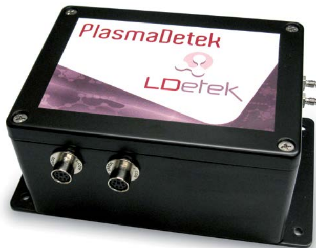
Figure 3: Plasma Detector module in the LD8000
