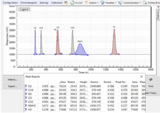
Chromatogram of trace ppm impurities O 2 -CH 4 -N 2 -CO-CO 2 -NMHC-H 2 in pure D 2 (deuterium)
