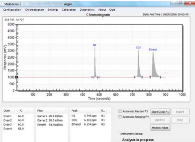
Span calibration chromatogram for Argon method:
