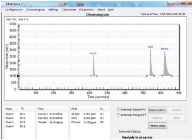
Span calibration chromatogram for Nitrogen method:
