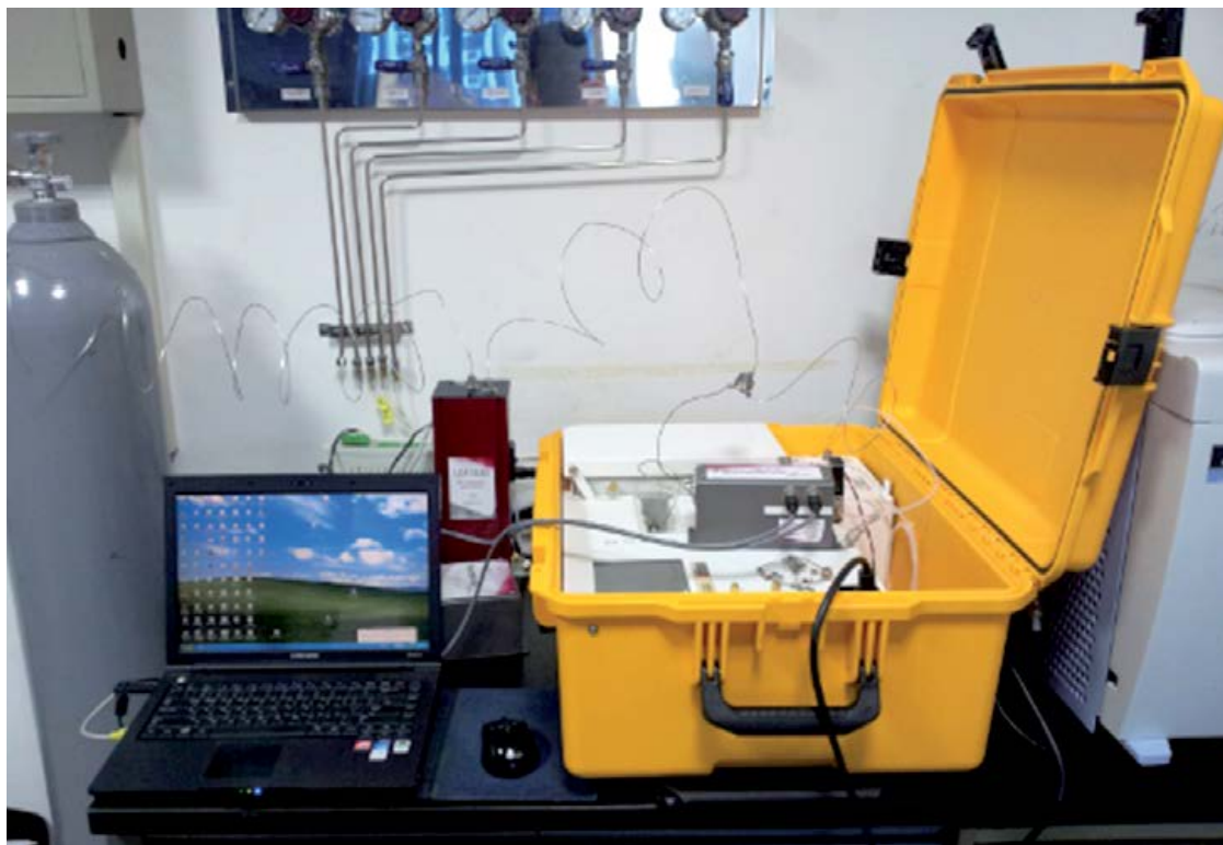
Figure 5: PlasmaDetek installed in a portable unit
