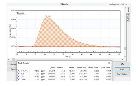
**Repeatability:** Based on the GC standards. Using 6 of 10 consecutive runs, being lower than 5% of 3\*CV%
