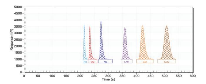
Chromatograms (Span calibration) of trace impurities H2-02-N2-CH4-CO-CO2 in balance gas Argon
